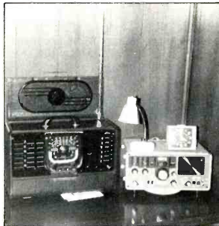
Richard Persinger of Michigan chases pirates with his 1948 Zenith transoceanic and Yaesu FRG-7 receivers.
